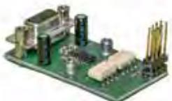
**EX-MS2****MODULO DI CONNESSIONE SERIALE RS-232**
