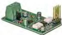
**EX-MS5****MODULO DI CONNESSIONE SERIALE RS-485**
