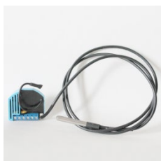
Temperature Sensor connection to the device
